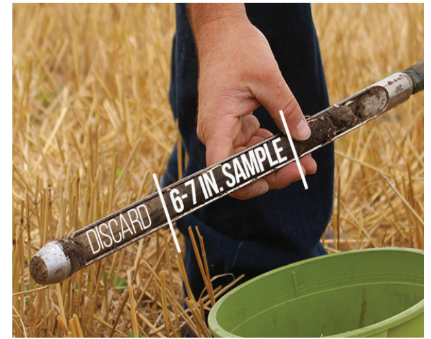
The photo above demonstrates the portion of a soil core necessary to create a proper soil sample.
